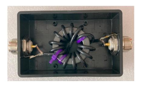
Mark the center of the coax with a bit of electric tape, and feed the coax through the toroid core so the mark is in the center of the toroid hole. Snug down (finger tight) a cable tie to hold the coax center in place - then loosely attach two more cable ties that will secure each coax end. Take one tail of the coax and begin winding turns, keeping the coax turns snug and neat against the toroid.
